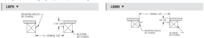
STEP 2: Lay core onto mounting angles.
