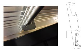
STEP 3: Keeping CCRT pulled up against the core clip, use the CCRT as a lever pushing against the core's spacer bar/mandrel tube to unclip core clip from bar.
